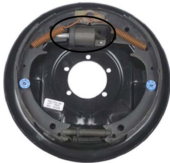
Hydraulic brakes: small cylinder circled.
